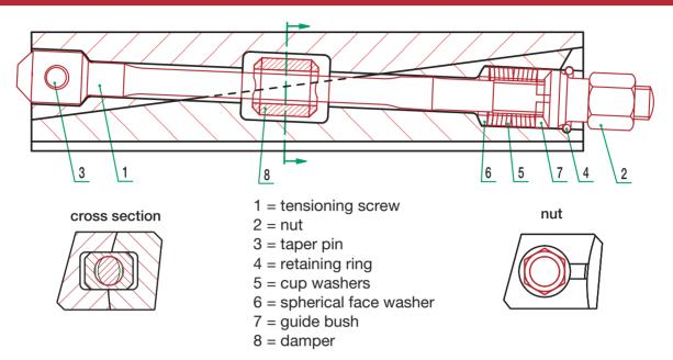
On the Feuerbacher tensioning keys "D" the tendency for vertical offsetting of the Feuerbacher tensioning key halves is taken up by a damping block. This is particularly valuable when clamping upper dies.
