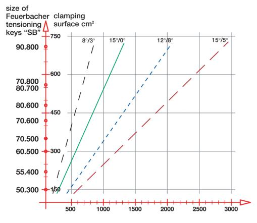
upper die weight in kg (approx.) for forging hammers or counter blow hammers
